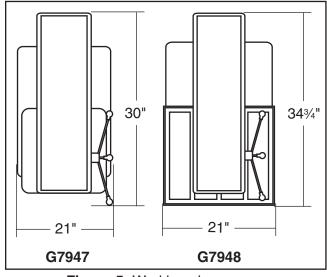
Figure 5. Working clearances.
